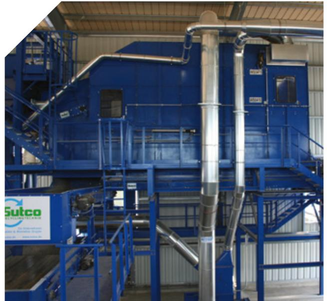
ted in a circulation air mode. A part of the sucked air is delivered to a dedusting unit so that the separation chamber is kept under vacuum and an escape of dust is largely prevented.
